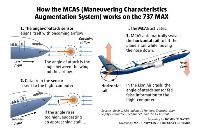
Figure 1. How the MCAS works on the 737 MAX (Nowlin, 2019)
