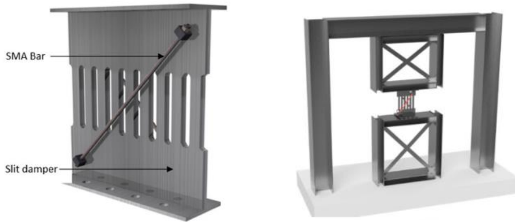
Figure 2-16. Configuration and installation scheme of steel slit-SMA hybrid damper [161]
