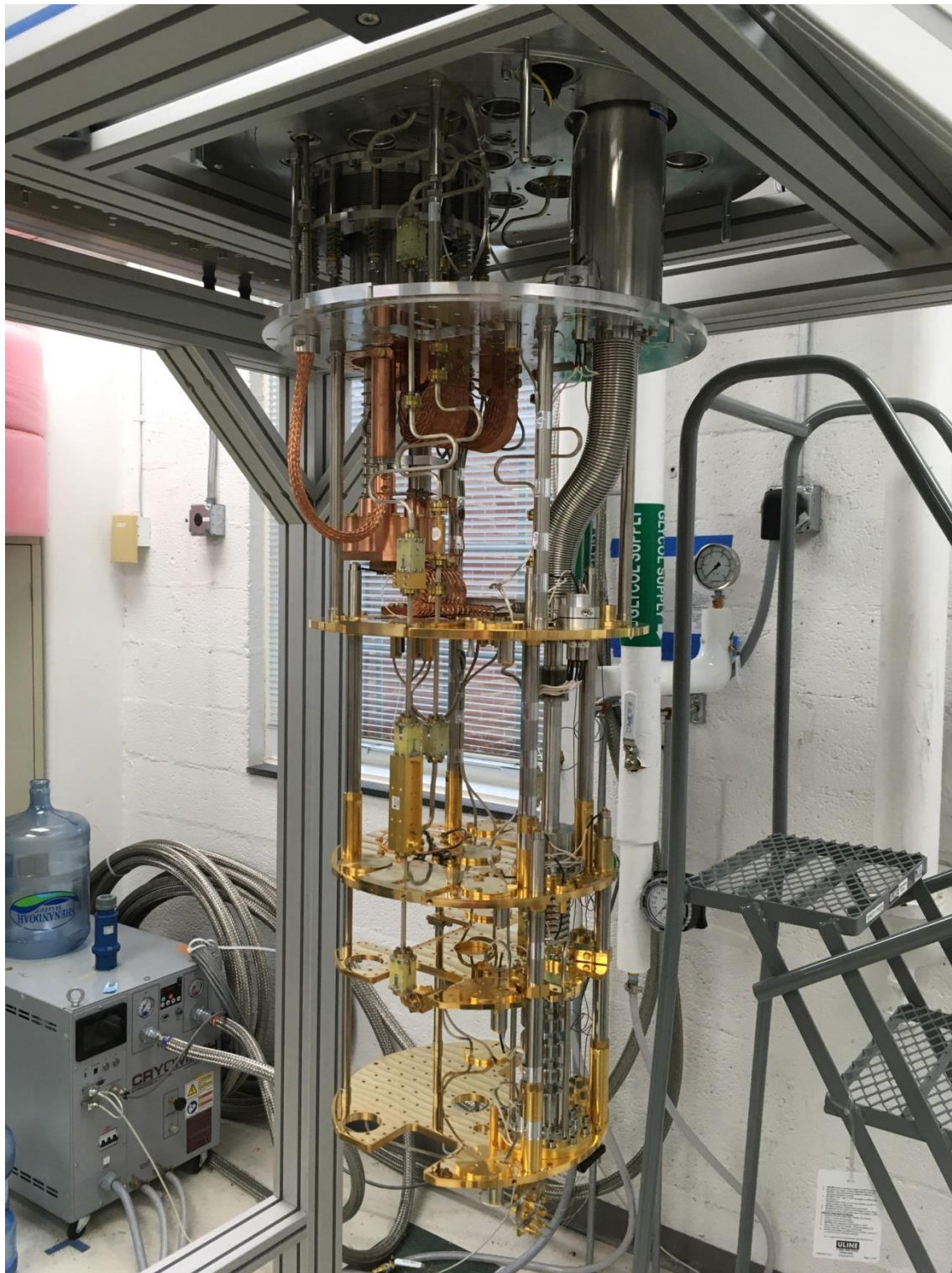
Figure 51: A picture of the open BlueFors cryostat with the w-band waveguide system installed.
